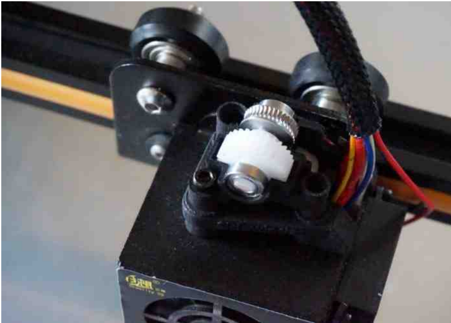
Fig. 7: Insert the gear shaft with bearings, then close with the top half of the Nimble Sidewinder
