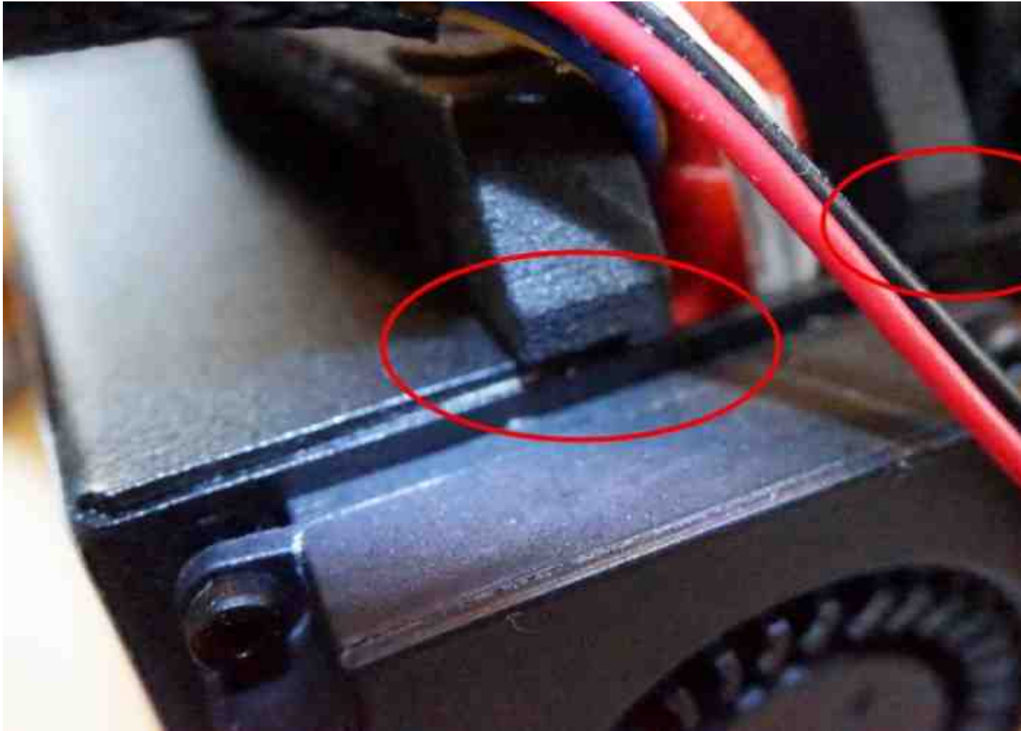
Fig. 2: Slide the mount block in sideways, making sure no wires are trapped on the right hand side.
