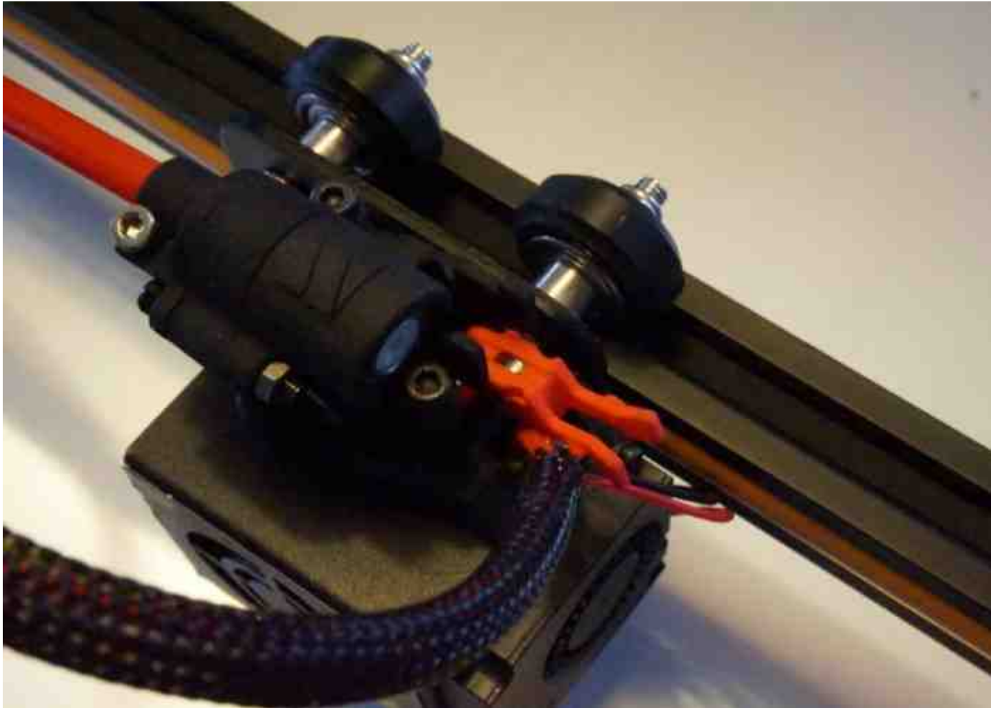
Fig. 15: Open the Breech block by squeezing the “ears” together.
