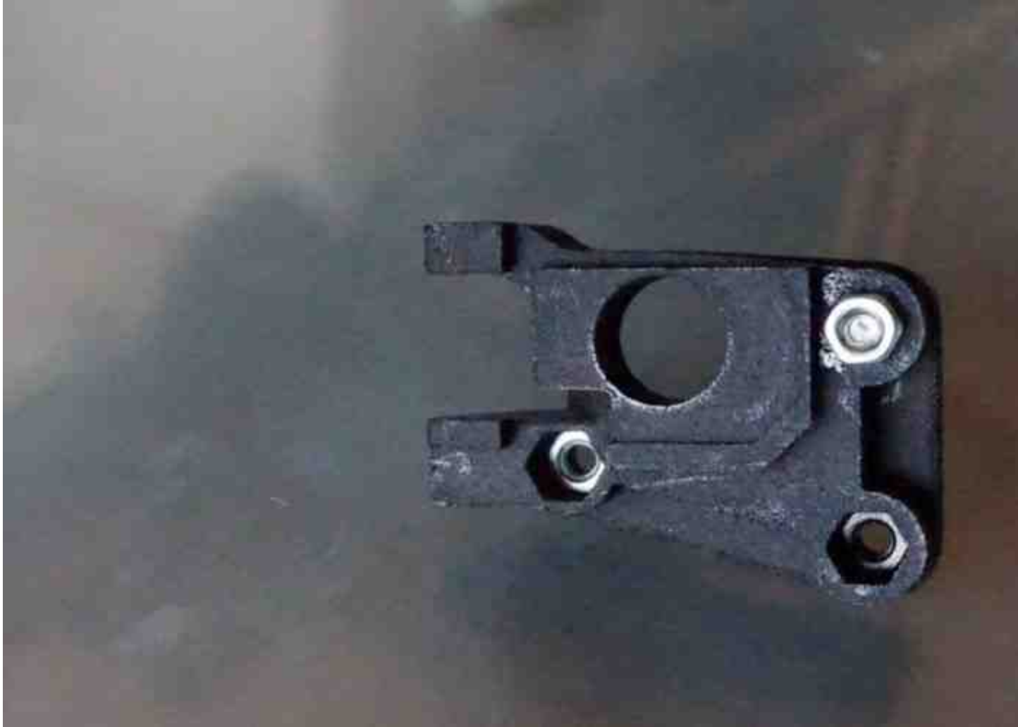
Fig. 1: Insert 3 x M3 nuts into the nut traps underneath the Nimble Sidewinder mounting block.
