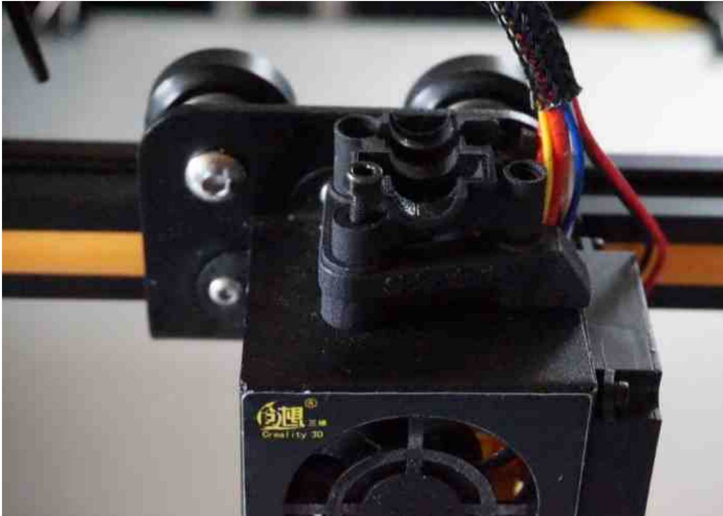
Fig. 6: Fit the Bottom half of the Nimble Sidewinder
