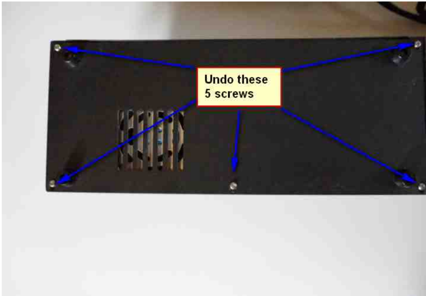
Fig. 11: Undo these 5 screws, take off the base plate and put it aside.
